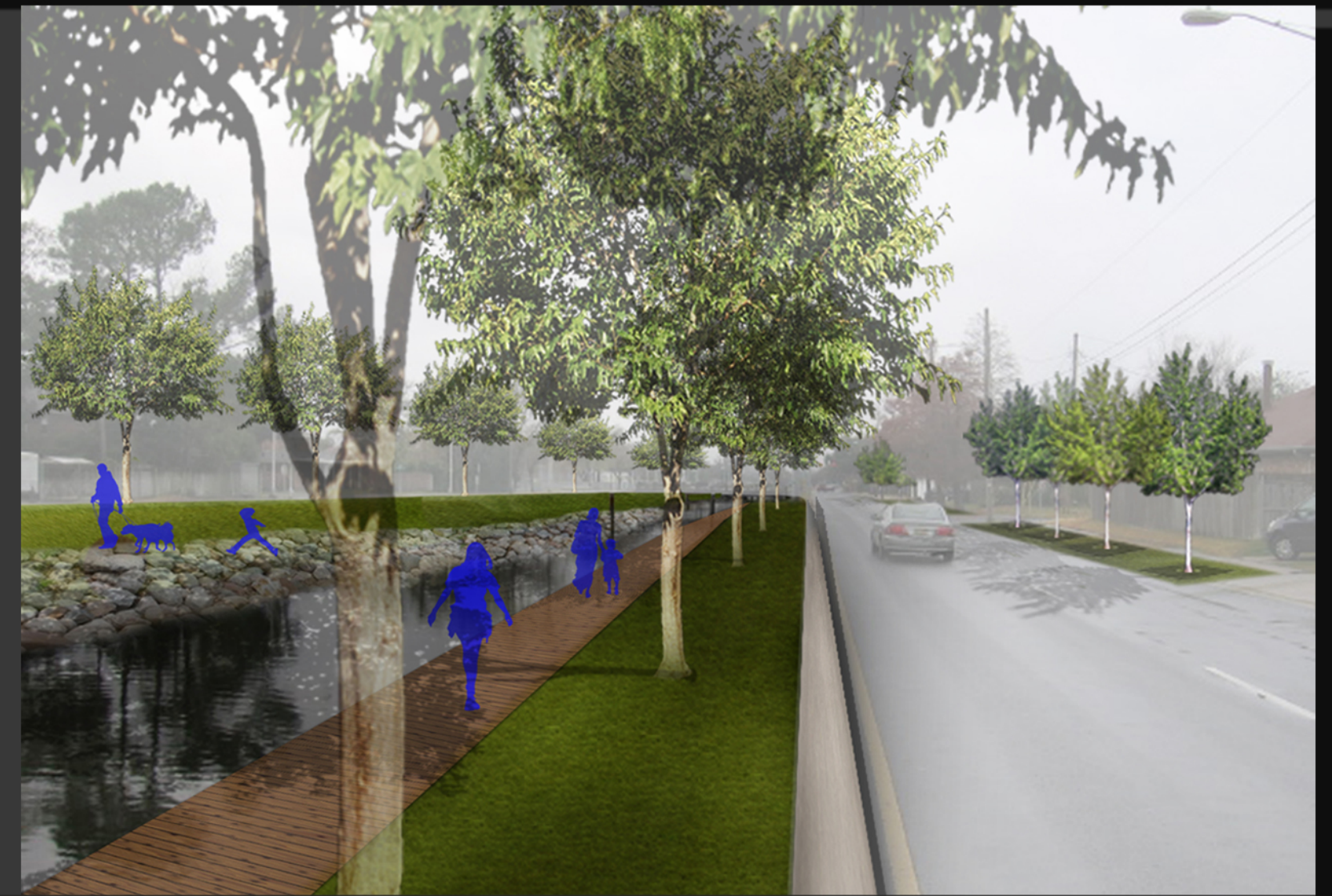
IN LIMITED BANK AREAS, BOARDWALKS WILL BE BUILT ONTO SIDE SLOPES AND CANTILEVER SECTION OF THE CANAL. THIS ALLOWS FOR STREET TREE, WETLAND PLANTINGS AND RIP RAP FOR SLOPE STABILIZATION.
