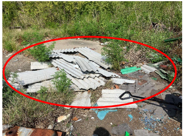
Photo of ACM building and construction debris.
