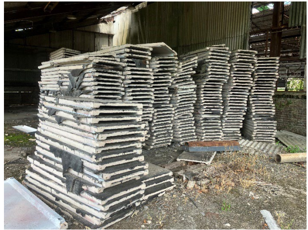
Photo of black tar on non-ACM cement panels stored in the Factory Building.
